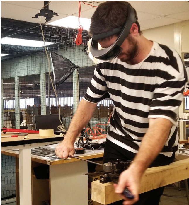
Figure 4. MR-assisted manual steel bending. Spatial Futures Studio.
